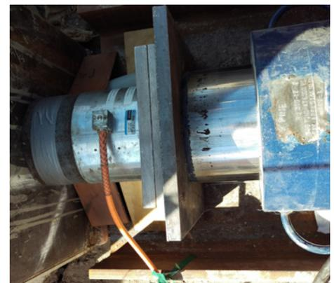
Lateral load test jack and load cell
